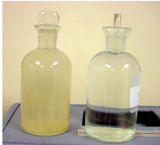
Figure 4-10. Phosphate precipitate (bottle on the left) which can cause milky water complaints.
