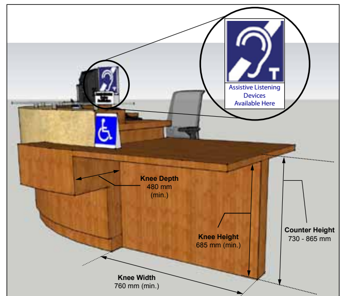
Figure 100: Dimensions of Accessible Service Counter
